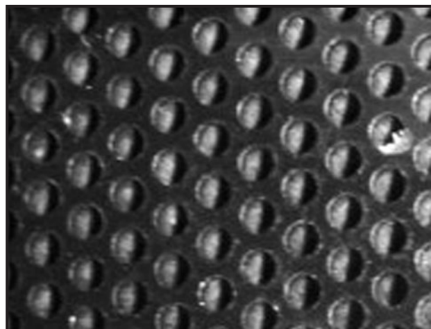
Figure 4.27: Photograph of a medium-energy collimator
