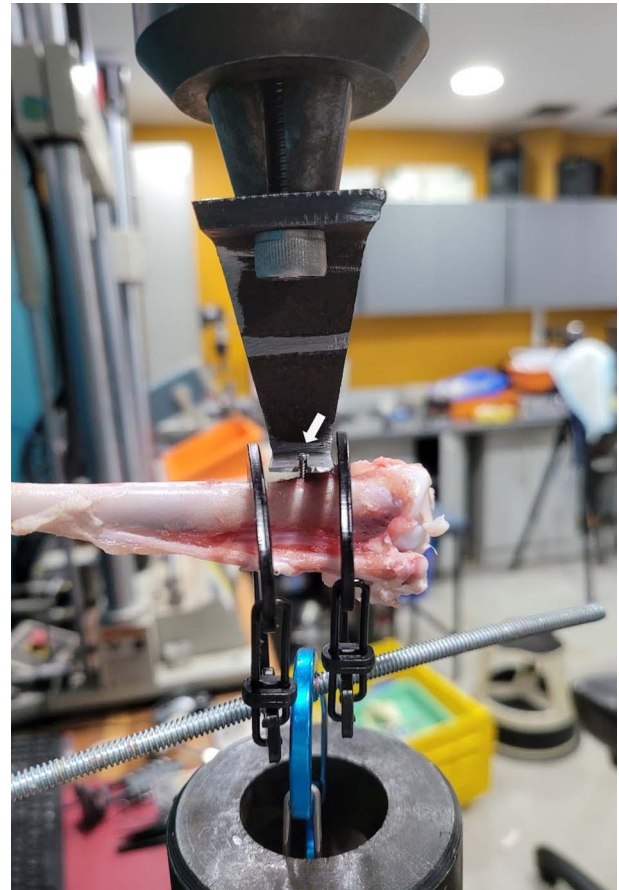
Figure 2. Tibiotarsus of a Pekin duck ( Anas platyrhynchos domesticus ) with 1.5-mm locking screw (white arrow), inserted mediolaterally, at the proximal metaphysis (location 5). The screw head is engaged in a custom-made testing jig prior to axial screw pullout testing with a servohydraulic testing machine.
